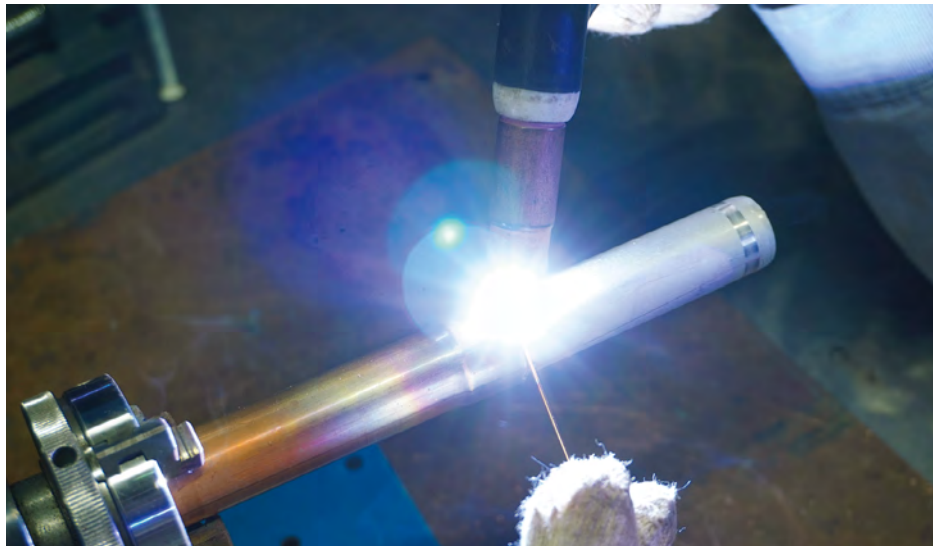
Welding copper and stainless steel using a copper-iron alloy
