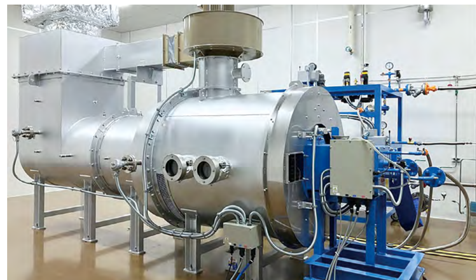
Mixed hydrogen combustion and oxygen-enriched combustion equipment at the Iwatani R&D Center
