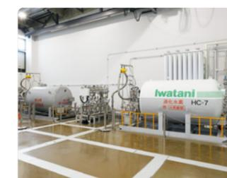
Testing equipment for liquid hydrogen
