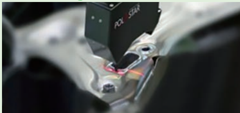
Automation of welding inspections
