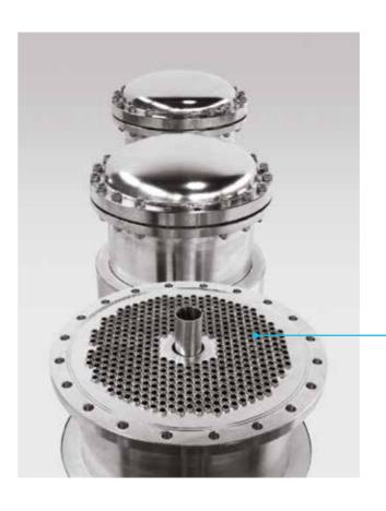
THE PIPES ARE EXPANDED INTO THE PLATES, AVOIDING ANY WELDING FOR A TOTALLY HYGIENIC EXECUTION, AND A BETTER RESISTANCE AGAINST DILATATION STRESS.
