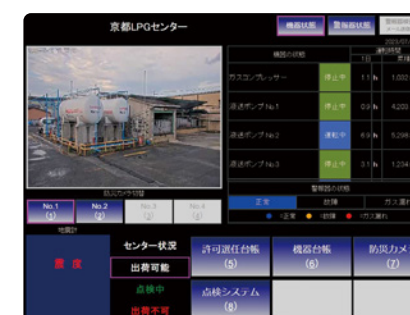
Using cameras to check on the state of damage through the safety system
