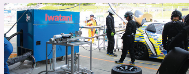
Liquid hydrogen filling equipment for the hydrogen-engine Toyota Corolla
