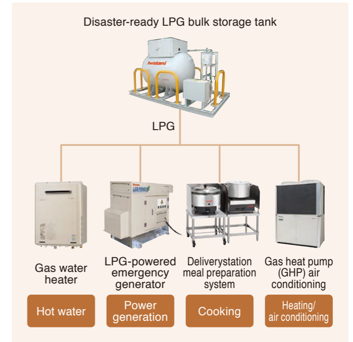
The Iwatani Emergency Energy System
